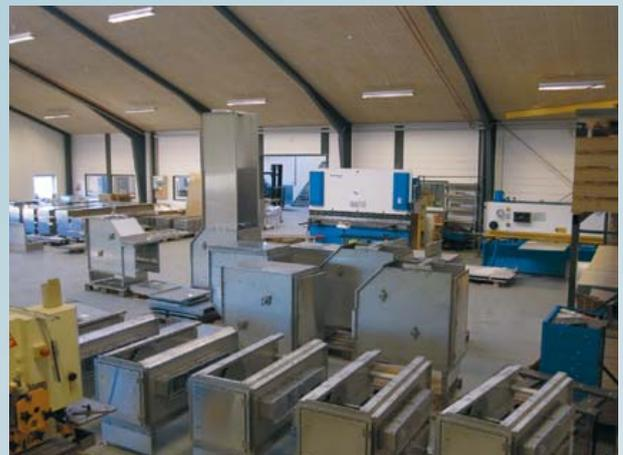
*Production of stainless elevators for conveying of enzymes.*
