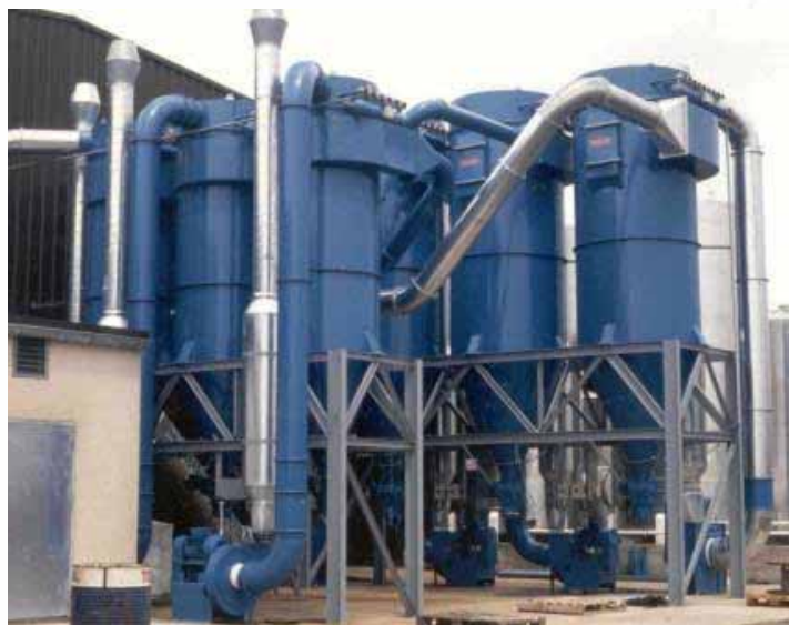
SimPact 4T pulse-jet filters collecting marble, glass, and polyester dust at S.T.D. plant in France
